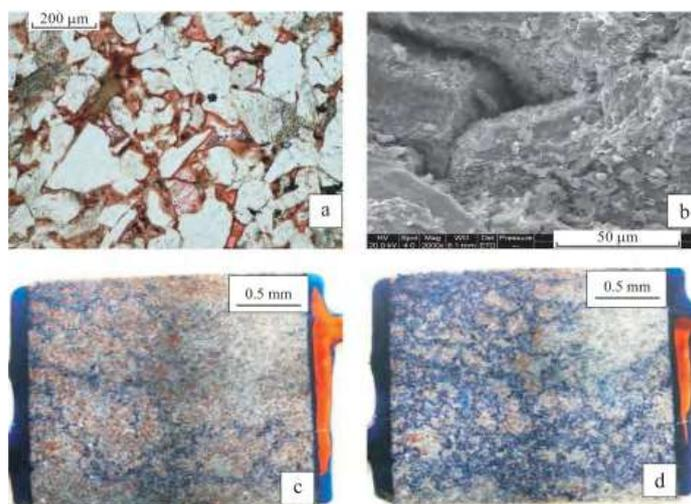
**Fig-1: Microscopic photos of remind intergranular pores (a, b) and water flooding with models of intergranular pore(c, d)**
