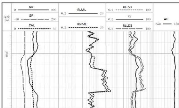
**Fig-4: Overlap diagram of resistivity calculated by apparent acoustic porosity and formation apparent resistivity response curves (poor fracture)**
