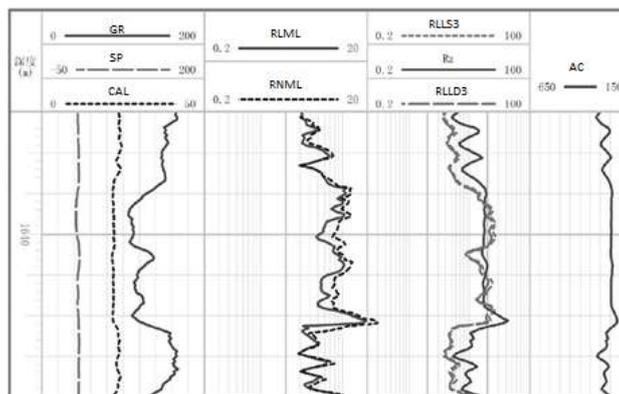
**Fig-3: Overlap diagram of resistivity calculated by apparent acoustic porosity and formation apparent resistivity response curves (fracture develops generally)**
