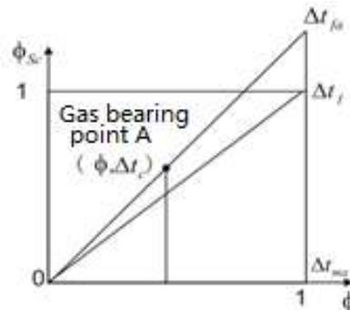
Fig-3: Cross plot of true porosity and acoustic porosity
