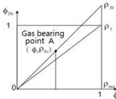
Fig-2: Cross plot of true porosity and density porosity
