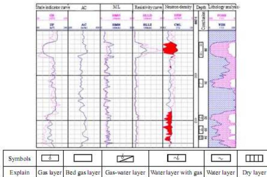
Fig-4: Well \*\*\* Gas bed coincidence curve recognition
