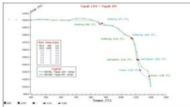
**Fig-3: Thermal microscope image of the industrially applicable opaque glaze**
