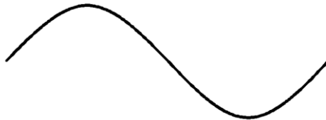
Fig-1: Change in curvature of an arc or curve from concave to convex
