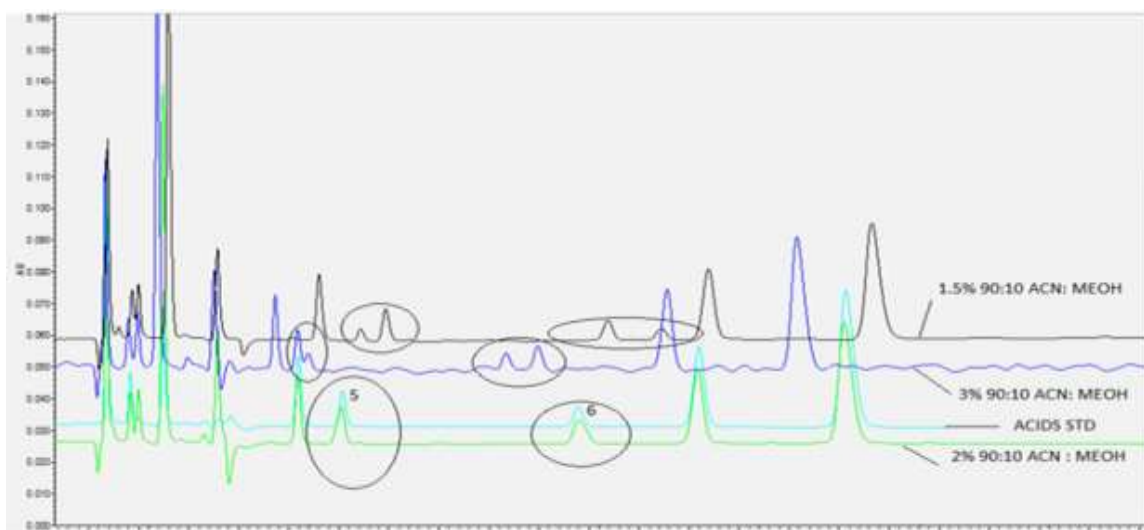
Fig-5: (D) Impact of mobile phase composition on the separation of organic acid peaks
